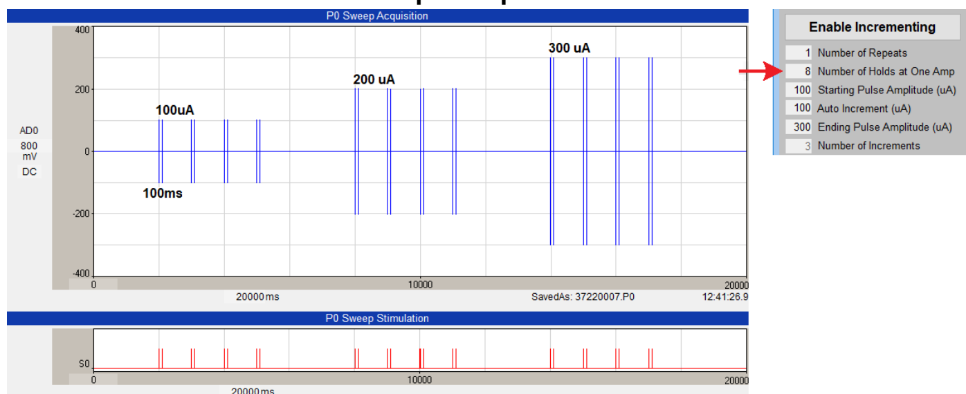
Fig. 3.4.2.1. Incrementing Paired-Pulse stimulation every 4 th paired pulse. For 100 ms pulse period here, that would be just like incrementing every 8 pulses, so the Number of Holds at One Amplitude would be = 8 (red arrow).
