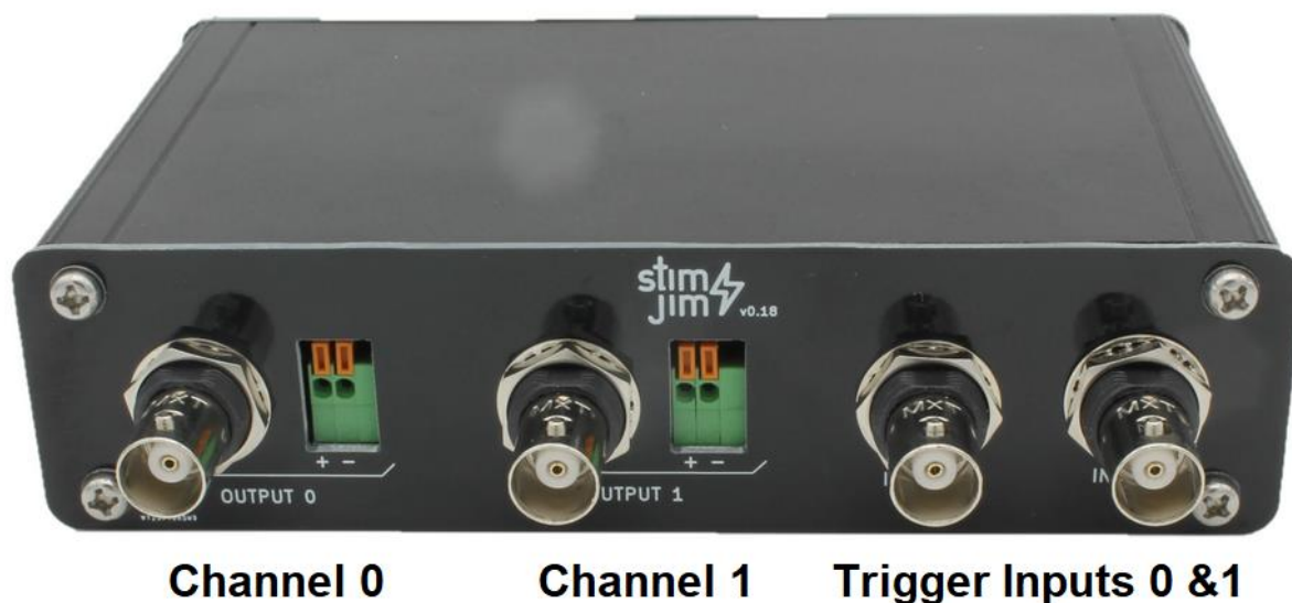
Fig. 1.3.1. The front panel of the StimJim showing Channel 0 and Channel 1 outputs (both a BNC connector and 2 + and – pins), and Input 1 and Input 2 BNC connectors.
