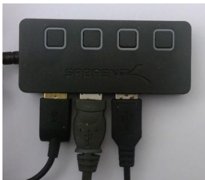
Fig. 2.2.2. Using a USB hub to connect to multiple StimJims.
