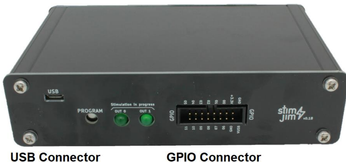
Fig. 1.3.2. The back panel of the StimJim showing the delicate USB Micro-B connector, the two green LED lights that illuminate when the StimJim is initially plugged into the computer and when pulses/trains are output, and the General Purpose I/O (GPIO) 16 pin connector.
